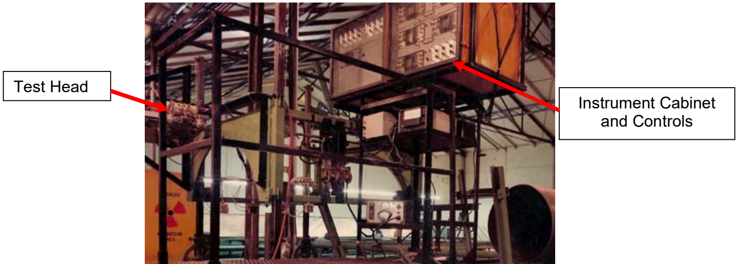
5 Channel Straight Seam DSAW Testing System.
