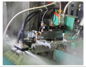
The view above shows a close up of the FG7200 Test Head with view of the Oscillator Bearing Assembly and the Probe Shoe assembly riding over the Hot Weld. This Flash Gauge is installed 3 meters downstream of Weld Pressure Rolls and 3 meters upstream of the Seam Annealers on a 14" API 5L Mill.
