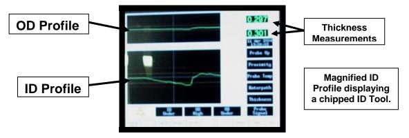
The Flash Gauge is installed immediately down stream of the welder, where the weld is still at an elevated temperature. The Probe/Shoe assembly oscillates across the hot Weld Area, taking approximately 1000 thickness readings per stroke. These thickness readings are then plotted and displayed on the operator's computer monitor.
