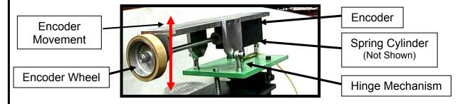
The Encoder and the mounting mechanism should be cleaned on a regular basis, simply because they are Electronic Components, and to ensure the Encoder wheel is allowed to move freely. The Encoders, at rest, should never be much more than 13mm (0.500") above the Pass Line of the Mill/Conveyer, as the
