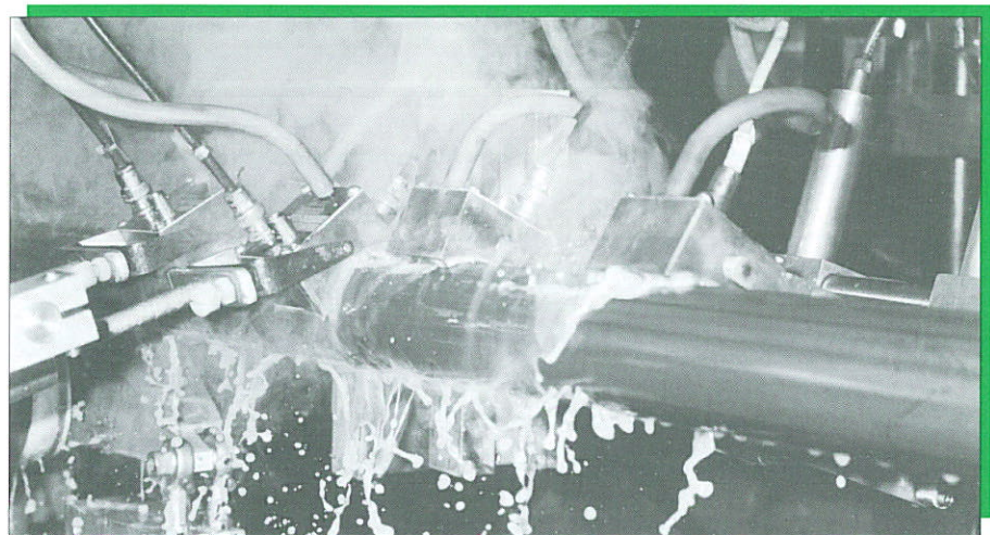
Four channel system – immediately after welding
