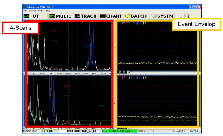
The Event Envelop is simply a Digital Chart Recorder, that show Defects that have been detected by the system. The Event Envelop operates in two ways, by time and by mill speed. The software changes the reference to Time, when the system is in Calibration Mode, and to Mill Speed (via the encoder) while the mill is running. The green highlighted area, in the Task Bar shows the speed of the mill based on encoder pulses.
