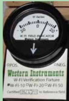
W-FI Magnetic Field Indicators Linearity Demonstration Kit. Illustrates linearity between 3 Models of W-FI's
