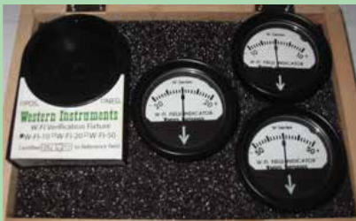
W-FI Magnetic Field Indicators Linearity Demonstration Kit. Illustrates linearity between 3 Models of W-FI's
