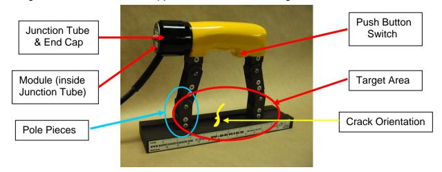
1. Solid State Push Button Switch – The Solid State Push Button Switch was designed for comfort and safety. While depressed, the switch delivers a ½ Watt control signal to the electronic controls (semiconductors) sealed in the Output Module. The Module connected to a receptacle plug in the Junction Tube of the Yoke, and supplies the necessary power (AC) to the coil encapsulated in the Yoke housing.
