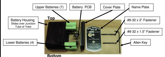
The 2 Battery sections are tabed, and are connected to the Battery Pack Printed circuit Board by the eyed Interconnection wires, Workman like care must be taken when replacing single cells, but can be easily performed by a battery service company. If the upper and Lower Battery sections are to be replaced, prewired ones can be ordered from Western Instruments. The picture below illustrates the position of the interconnection wires on the Battery Printed Circuit Board.
