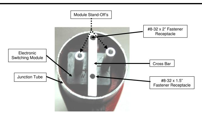
The Module is fitted with 2 Stand-Off's (Aluminium or Brass) that permit the connections to the Module to the Printed Circuit Board. If these fasters are over tightened, the Module can be pulled from the Molex Connector inside the Junction Tube. If this has occurred, a rigid rubber spacer (like a yellow Switch Cover) needs to be placed between the Module and the Cross Bar, which will keep the module Pressed into it's connector.
