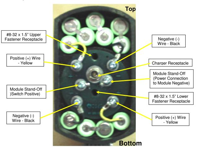
If the Battery is assembled in reverse (4 cells at the top instead of the Bottom), and the connections for the Module Stand-Off's are forced to make the screw connection, total failure of the Module will occur. Furthermore, one or more of the AA NiMH Cells may fail due to a short circuit.
