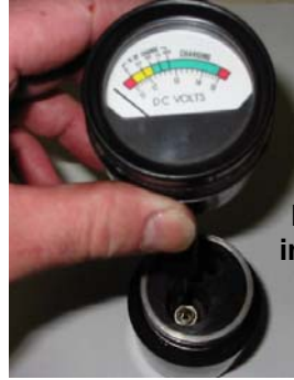
Battery Meter measuring Battery under load.
