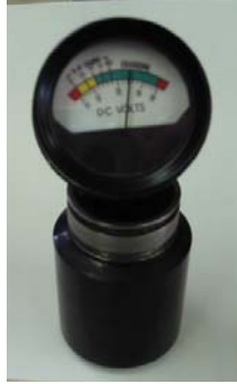
Battery Meter measuring Battery under load.
