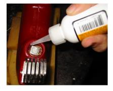
Applying glue carefully on switch cover Seat
