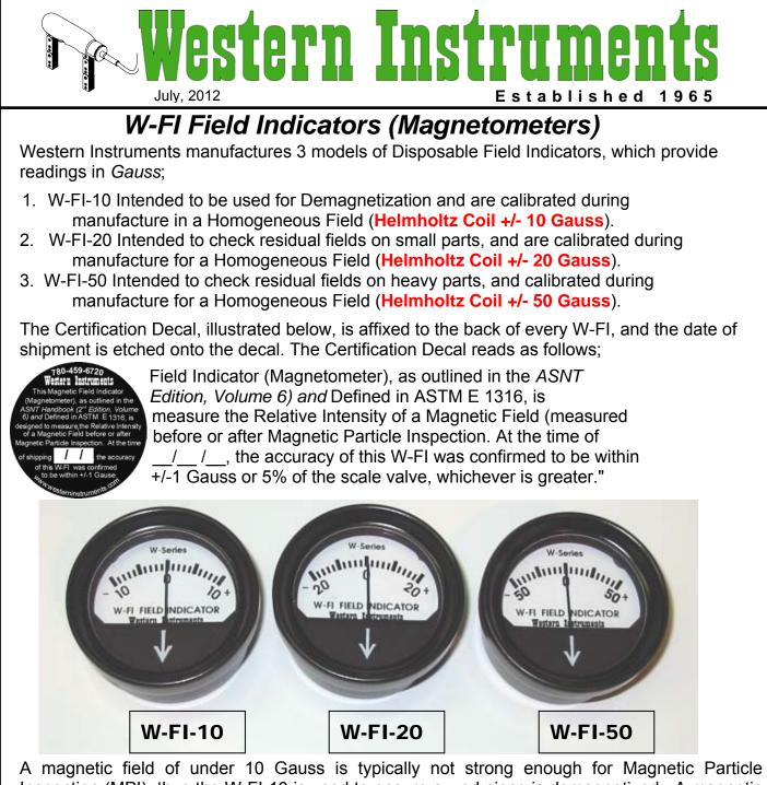
A magnetic field of under 10 Gauss is typically not strong enough for Magnetic Particle Inspection (MPI), thus the W-FI-10 is used to ensure a workpiece is demagnetized. A magnetic field, for MPI, should be approximately 18 to 24 Gauss, thus an inspector uses the W-FI-20 to ensure his field is strong enough. A workpiece can be magnetically saturated prior to or after inspection, and these strong fields are evaluated with a W-FI-50.
