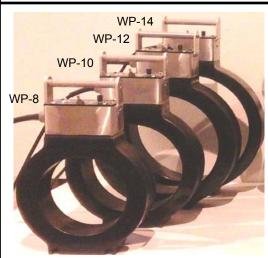
Western Instruments new Medium Duty WP-Series of Portable MPI Coils are a completely new platform. They are not based on any existing type of Coil, having been developed from Customer input and using our advanced Electro-Mechanical Engineering. WP-Series Coils are being offered in 4 different ID Sizes; 8" (203mm), 10" (254mm), 12" (305mm) and 14" (355mm), and have been appropriately named; WP-8, WP-10, WP-12 and WP-14.
