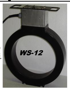
WS-Series Coils provide a powerful DC Pulse, once per second from a our CD (Capacitive Discharge) Power Supply. While the WS-Series uses a similar Coil Housings to Our WA and WP-Series Coils, it is slightly taller, built with a top panel with convenient handles. WS-Series Coils are completely different due to the unique CD Spike Power Supply for a field that extends into box end threads.
